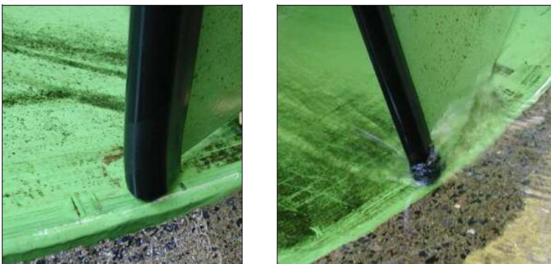
Figure 4: images of the leading edge of a screw, fitted with a rubber bumper
