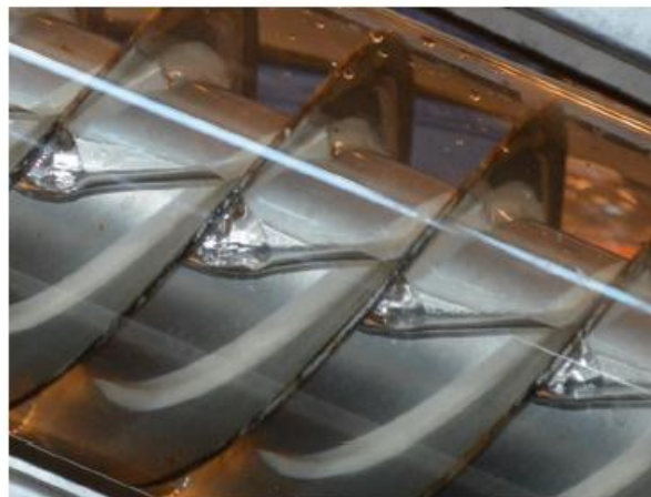
Figure 3. A laboratory-scale Archimedes screw. Gap leakage is visible across each flight where the lower bucket water level is below the leakage point, however gap leakage is occurring around the entire wetted perimeter of the flights.
